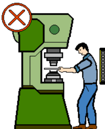
insertion between the barrier and dangerous zone
